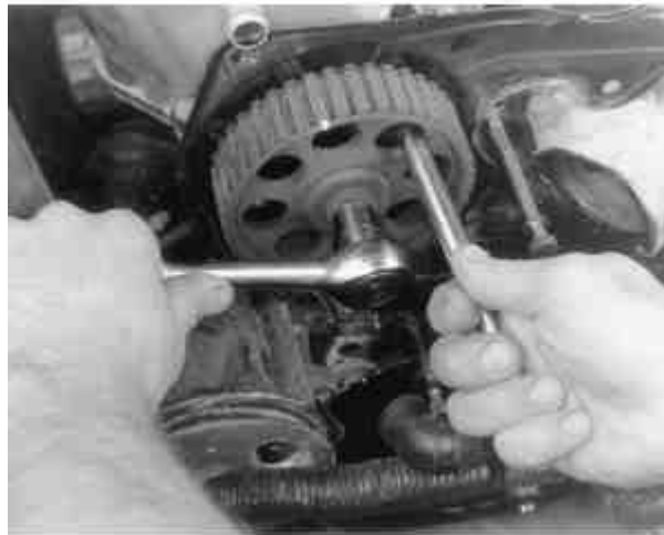
Fig. 3: Remove the camshaft pulley retaining bolt
